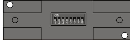
1. Termination resistors for RS485 master;
