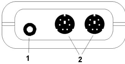
1. **Output:** Operation as interface: Connect to optically isolated interface adapter (accessory: GRS 3100, GRS3105 or USB3100)
