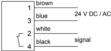
The switching outputs are self-configuring, depending on whether they are connected as PNP or NPN switches.
