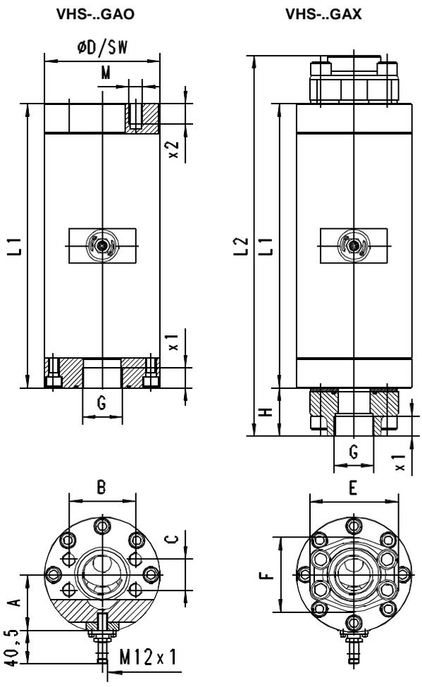
**SAE adapter for convenient installation and for increased stability to pressure! (350 bar)**
